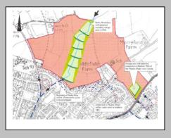
Added together these have provided a flow rate for run off to calculate the potential for mitigation of future flooding downstream. In summary, the Hailey Road stream culvert is too small, at only around two thirds of the capacity required. This means that a series of mitigation measures are required to store surface water in a cascade system on the site taking up approximately 6 hectares in order to limit the discharge flow rate from the land to the drain downstream of the culvert.
